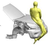
Autonomous vehicles will bring significant comfort benefits to passengers. However, safety cannot be compromised for alternative seating positions. Human Modeling and Simulation is currently the only technology that will allow assessment of occupant protection for new car interior architectures with flexible seat arrangements.
